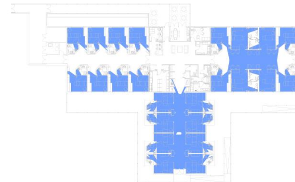
D. Visibility from each bedroom (patient's bed head), showing the different spatial properties between the three clusters.
